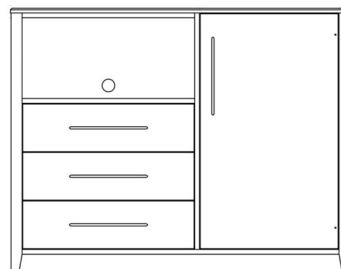
TG-0823G Microfridge.....54 x 22 x 42 Microwave Opening: 27 3/8 W x 21 3/8 D x 12 13/16 H Microfridge Opening: 22 1/8 W x 21 3/8 D x 36 3/4 H TG-0823R Microfridge w/Door...54 x 24 x 42 Microwave Opening: 27 3/8 W x 21 7/8 D x 12 13/16 H Microfridge Opening: 22 1/8 W x 21 7/8 D x 37 1/2 H
